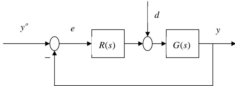
dove  $R(s) = \frac{(s+1)^2}{s^2 + 1}$  e  $G(s) = \frac{\mu}{s}$ ,  $y^0(t) = \sin(t)$ ,  $d(t) = \text{sca}(t)$ ,  $\mu > 0$ .
