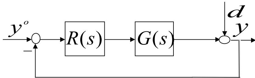
$$\text{dove } G(s) = \frac{1 - 0.5s}{s(s+1)}, \quad y^o(t) = sca(t), \quad d(t) = \sin(0.05t).$$
