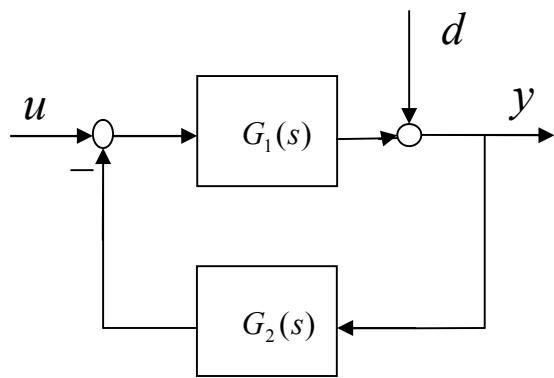
$$\text{dove } G_1(s) = \frac{1}{s}, \quad G_2(s) = \frac{8-s}{s+10}, \quad u(t) = sca(t), \quad d(t) = ram(t).$$
