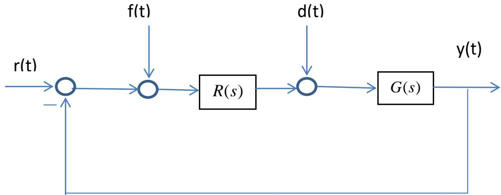
dove  $G(s) = \frac{1}{s}$ ,  $f(t) = \sin(t)$ ,  $r(t) = \text{sca}(t)$ ,  $d(t) = \text{sca}(t)$ .
